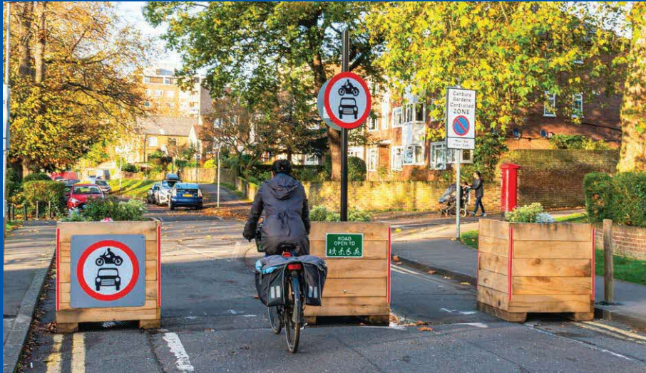
Modal filters on a road in Kingston upon Thames, one of the boroughs with LTNs.
